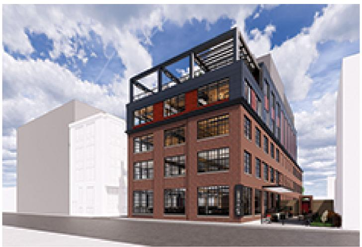
South Boston, MA Margulies Perruzzi (MP), along with Commodore Builders and structural engineer McNamara Salvia, have utilized cross-laminated timber (CLT) to add two stories to an existing 1920's era brick and beam building at 69 A St., creating a five-story 45,000 s/f building which is a hybrid of historical and new construction. MP navigated the complex permitting process on behalf of its client, and the building has been designed to accommodate either a single tenant or multiple tenants.
