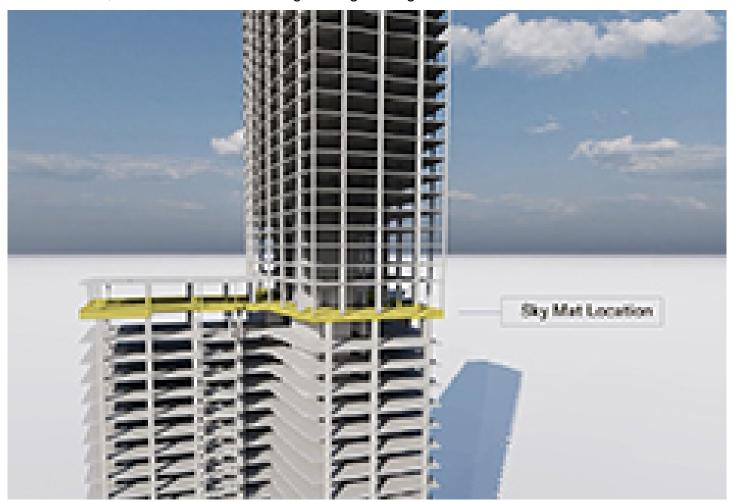
Boston, MA On a construction project site, a concrete pour in a deep hole or at ground level can be a complex logistical challenge requiring methodical planning and great attention to detail during execution. A recent concrete pour at Winthrop Center was no different – except that it occurred 350 feet off the ground.
